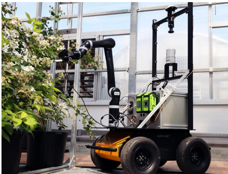
Slika 8. Robot polinator kupina (Izvor: https://www.wired.com/story/robotic-pollinator/ )
