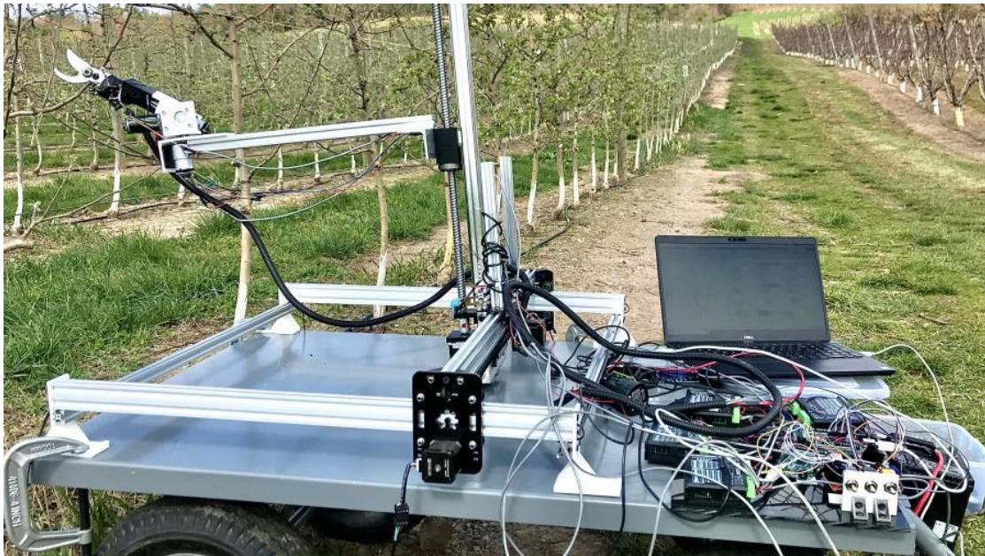
Slika 19. Robotski rezač Sveučilišta Penn State (Izvor: <https://www.growingproduce.com/fruits/robotic-pruner-ready-to-cut-down-production-problems-in-apple-orchards/>)
