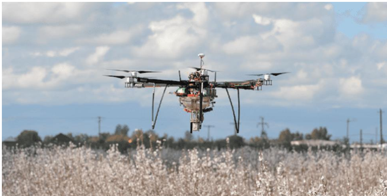
Slika 5. Oprašivanje voćaka iz zraka dronom (Izvor: https://fruitgrowersnews.com/article/new-york-invests-drone-pollination/ )
