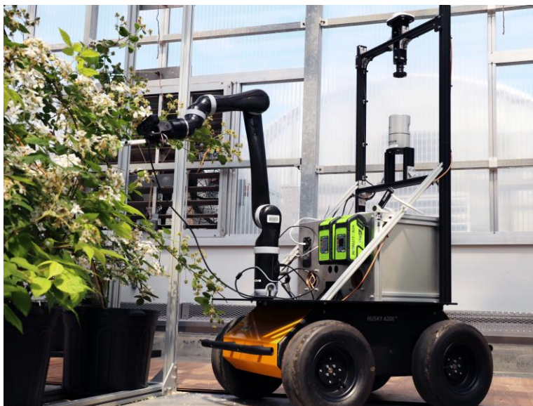
Slika 8. Robot polinator kupina (Izvor: https://www.wired.com/story/robotic-pollinator/ )
