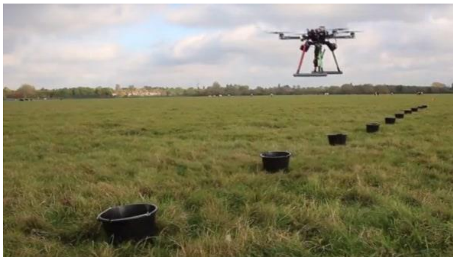
Slika 27. Primjer bespilotnog zrakoplova i način sjetve(Izvor: https://www.fastcompany.com/40450262/these-tree-planting-drones-are-about-to-fire-a-million-seeds-to-re-grow-a-forest )
