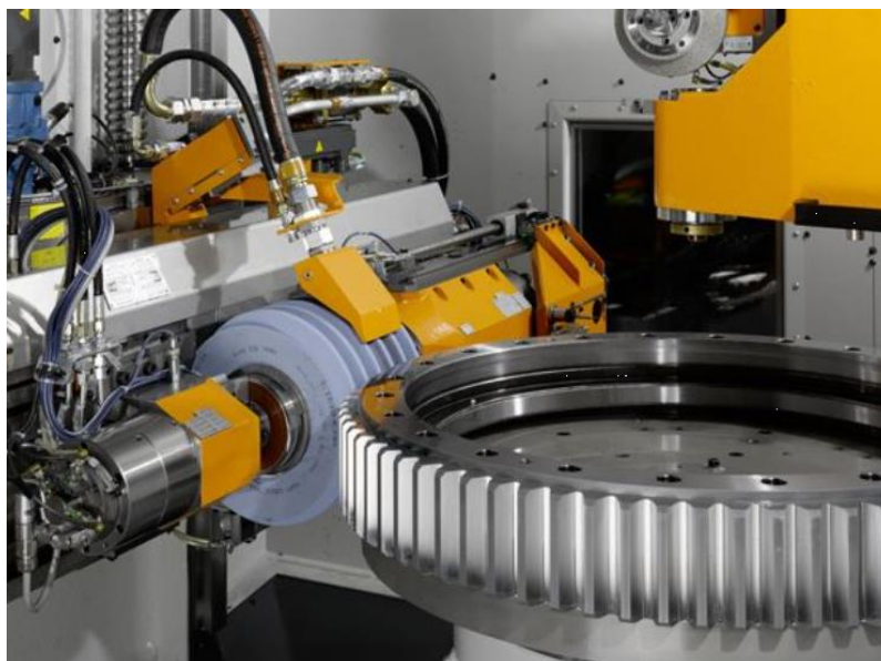
Slika 24. Precizno brušenje zupčanika (Izvor: http://hr.lemo-machining.nl/Content/ue/net/upload1/Other/134329/6361428886624032468094443.png )
