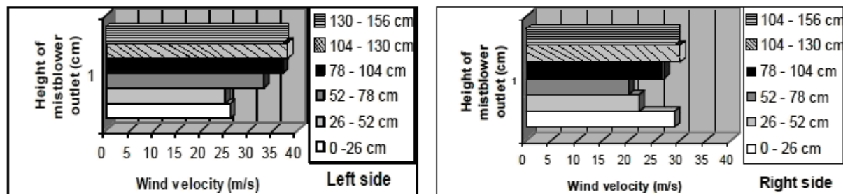
Figure 9. Distribution of wind velocity at different levels of the Hardi mistblower
