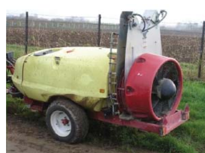
Figure 3. Mistblower (C) Hardi Zatum 1500
