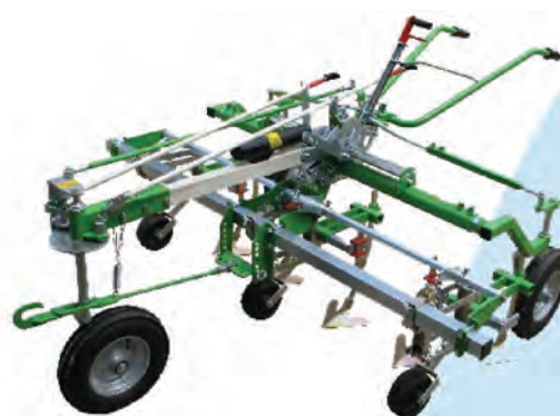
Figure 1. Newly developed inter-row cultivator
