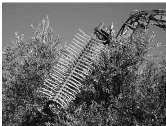
Figure 5. Rotor for fruit detachment
