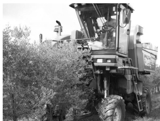
Figure 8. Overrow harvester for hedgerow olive orchards
