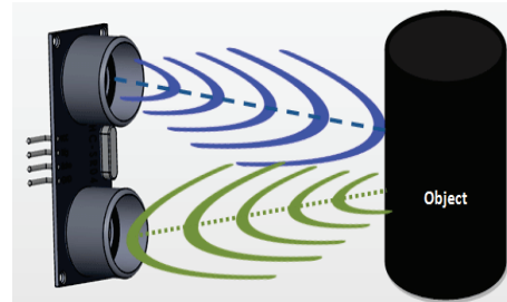
Figure 1 Ultrasonic sensor (Source: https://components101.com/ultrasonic-sensor-working-pinout-datasheet )
