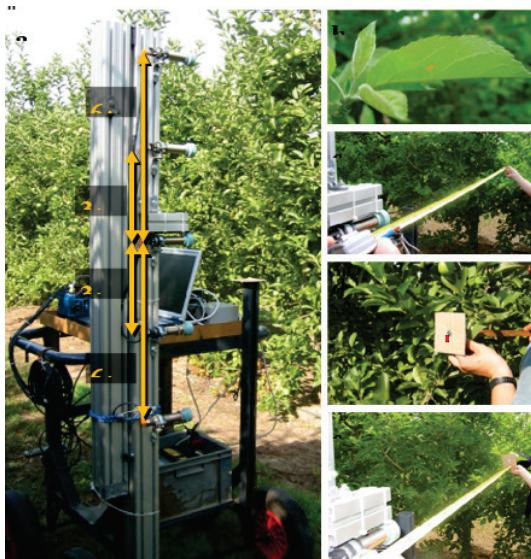
Figure 4 Test platform with ultrasonic sensors [42]
