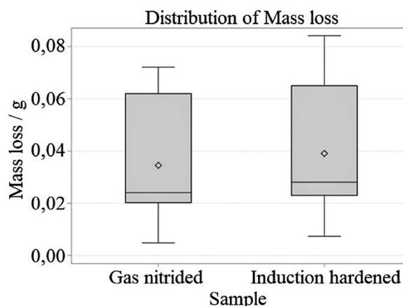
Figure 6 Distribution of mass loss depending on material condition
