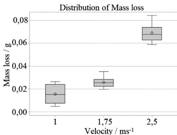
Figure 4 Distribution of mass loss depending on sample velocity
