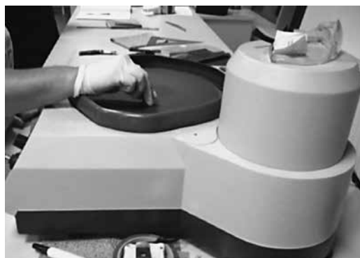
Figure 7 Machine polishing of plugs
