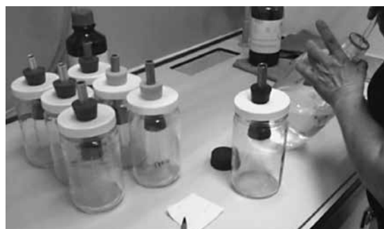
Figure 10 Extraction of glycerine solution from a jar
