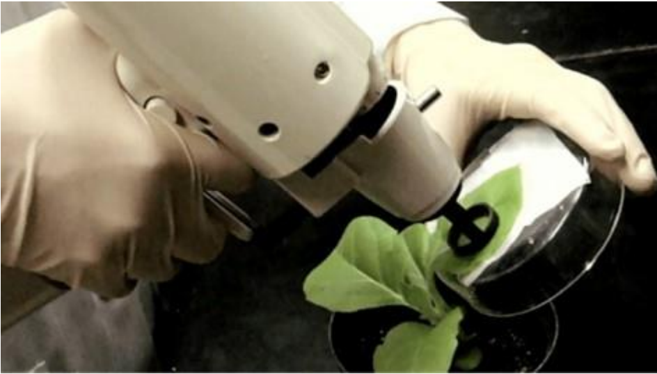
Fig. 5.4. Agracetus. Photograph of a gene gun. “Gene Gun: The Tool That Revolutionized Plant Breeding . . .,” by Matthew Wilde, 1 Mar. 2021. Genetic Literacy Project , geneticliteracyproject.org/2021/03/01 .
