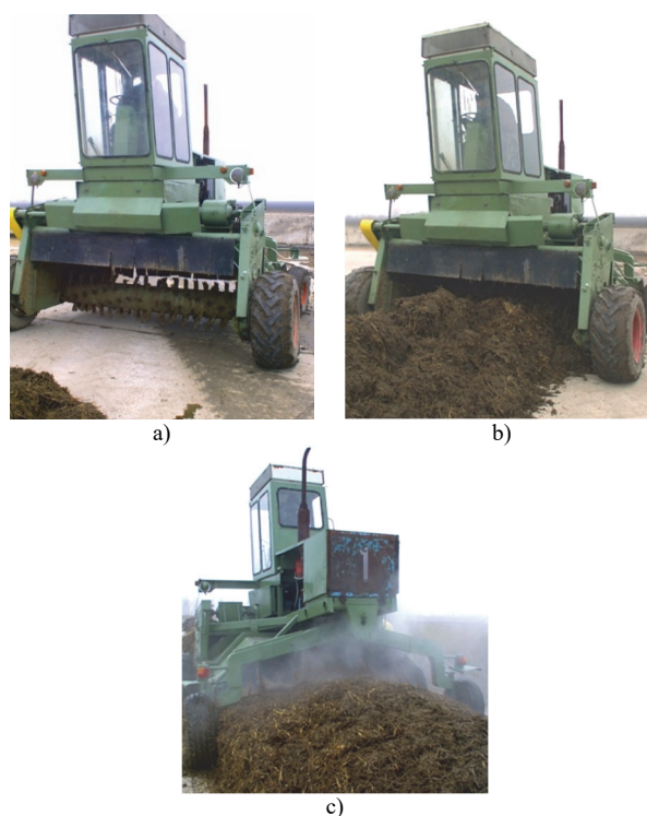
Figure 1 The self-propelled machine Kompomat 1: (a) prototype view; (b) untreated (raw) pile; (c) machine in work pile treatment
