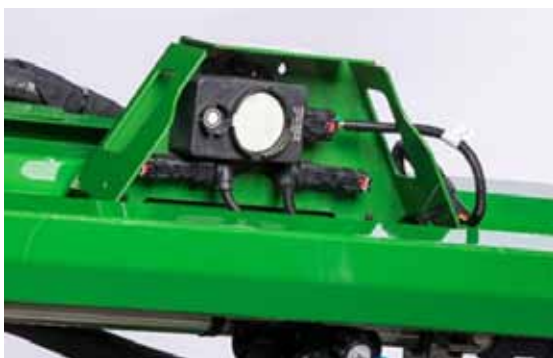
Slika 10. John Deere BoomTrac Pro senzor (Izvor: https://www.plattevalleyequipment.com/blog-news/sprayer-performance-upgrade-kits/ )
