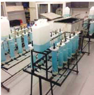
Figure 1. Experimental setup for anaerobic batch co-digestion of camelina and cow manure.
