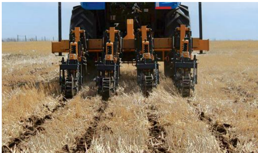
Slika 4. Strip tillage – obrada i sjetva u trake (Izvor: https://www.grainews.ca/crops/lets-talk-strip-tillage/ )
