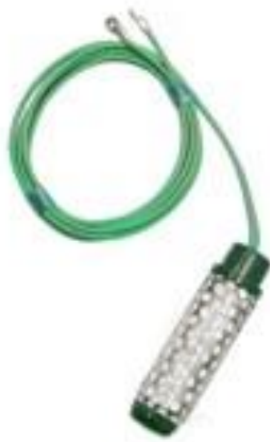
Slika 3. Granular matrix sensor (Preuzeto sa: http://www.irrometer.com/sensors.html )
