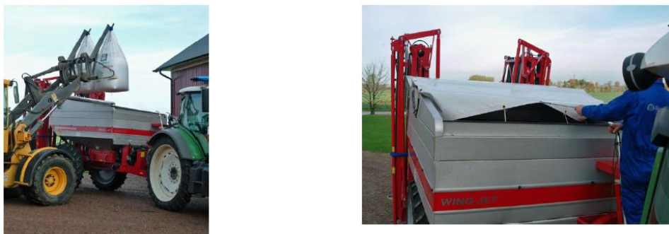
Slika 53. Punjenje rasipača Kongskilde Owerum Wing Jet K-plus Hidro S 4024 (Izvor: http://www.kongskilde.com/sv/sv-SE/Agriculture/Soil/Fertilising%20technique/ )
