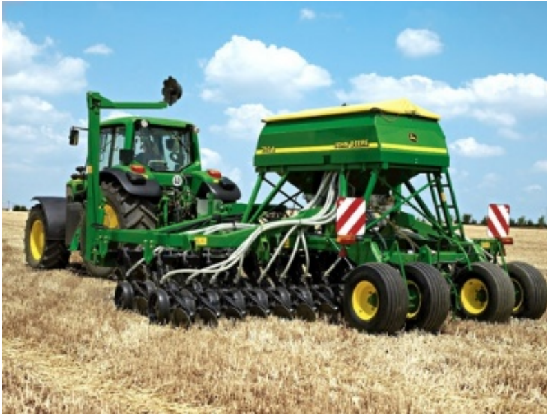
Slika 7. Pneumatska sijačica za žito No-till 750A 6m ( http://www.cerealsevent.co.uk/press-releases/john-deere-drills-work-in-all-conditions )
