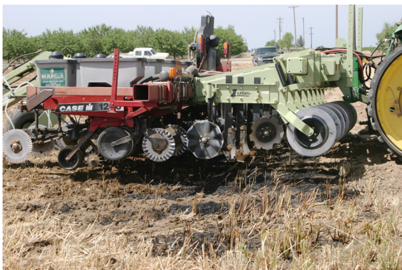
Slika 10. Orthman 1 tRIPr strip tiler i sijačica ( http://casi.ucanr.edu/files/43649.pdf )
